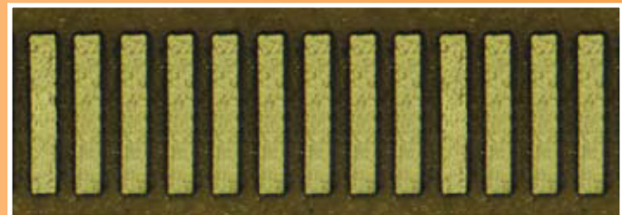
.001" thick Kapton webs are .003" between cutouts
