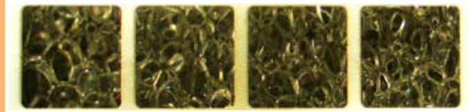
.020" thick 96% alumina webs are .010" thick with no signs of microfracturing or stress
